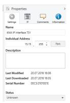
Within the "IP" overview the IP network specific options of the KNX IP Interface can be changed.
