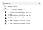
Each individual KNX address can be changed by clicking on the list entry and typing in the desired address into the "Individual Address" text-field. If the text-field frame switches to color red after entering the address, the address is already taken within your ETS project.
